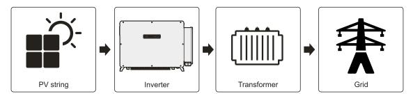
Figure 2-1 PV grid-tied generation system
