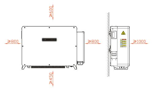
Figure 3-4 Installation clearance
