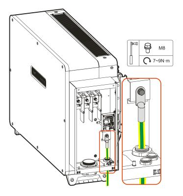
Figure 3-34 Connect internal grounding cable
