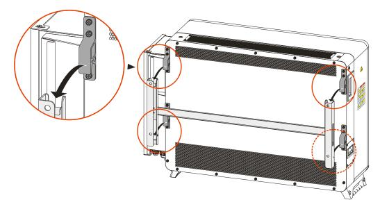
Figure 3-16 Hang the inverter onto the installation holder
