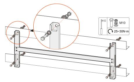
Figure 3-15 Fix installation holder
