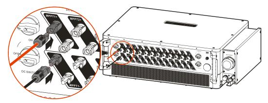
Figure 3-43 Connect PV connectors
