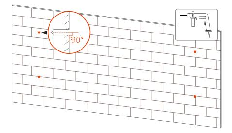
Figure 3-21 Drilling holes
