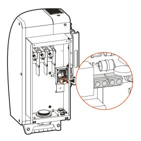
Figure 2-11 RS485 communication interface diagram
