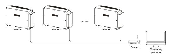
Figure 2-10 Ethernet monitoring (multiple inverters)
