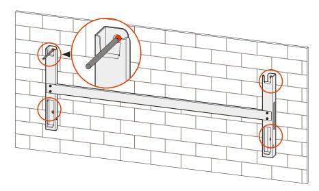
Figure 3-19 Mark the mounting holes position
