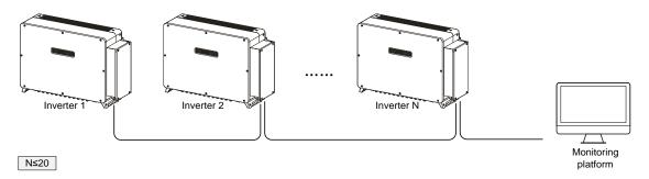
Figure 2-12 RS 485 communication (multiple inverters)
