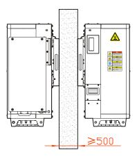
Figure 3-6 Back-to-back installation space requirements (unit: mm)
