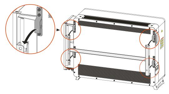
Figure 3-24 Hang the inverter onto the installation holder
