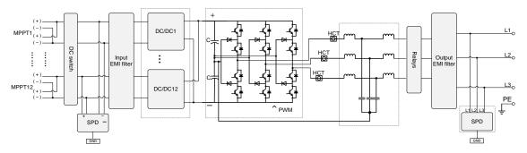
Figure 2-8 Working principle diagram
