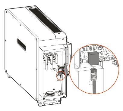
Figure 3-46 Ethernet communication connection
