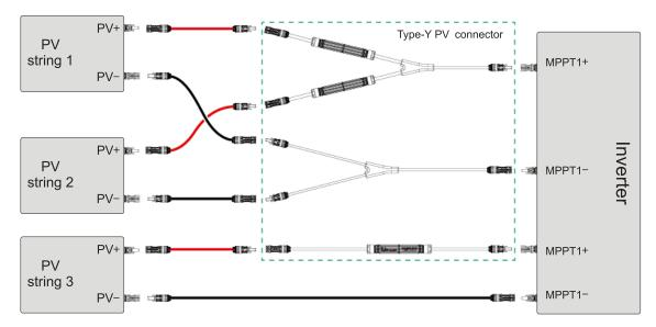
Figure 3-39 Wiring diagram (connected from inverter side)
