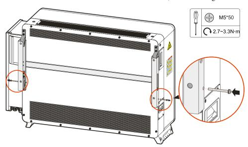
Figure 3-25 Fix inverter
