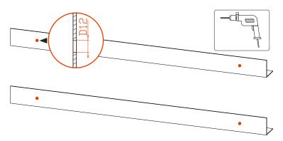
Figure 3-14 Drilling holes (unit: mm)
