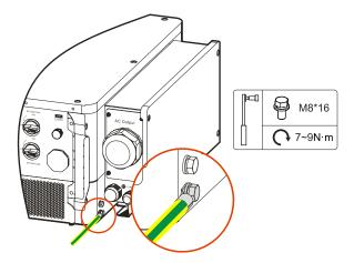
Figure 3-27 Schematic diagram of the ground connection
