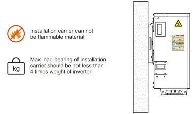
Figure 3-7 Installation carrier requirements
