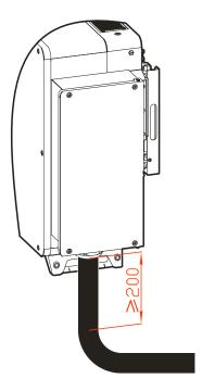
Figure 3-33 AC cable entry requirements (unit: mm)
