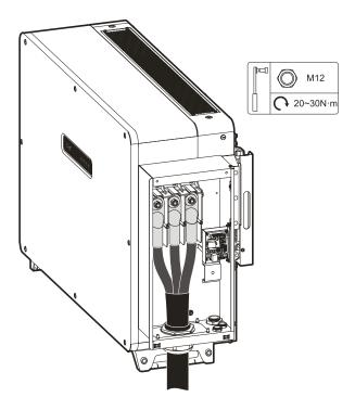
Figure 3-32 Connect the AC output cable
