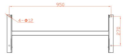
Figure 3-20 Mounting hole size(unit: mm)
