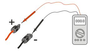
Figure 3-42 Measuring open-circuit voltage
