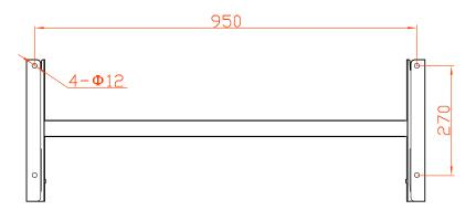
Figure 3-13 Mounting hole size (unit: mm)
