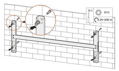
Figure 3-23 Fix the installation holder
