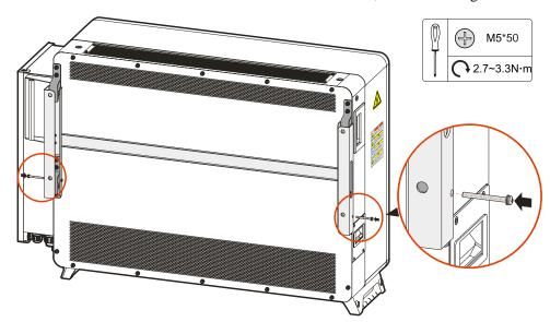
Figure 3-17 Fix inverter
