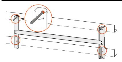
Figure 3-12 Mark the mounting holes position
