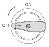
Figure 3-41 Diagram of DC switch OFF status
