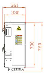
Figure 2-7 Size (unit: mm)
