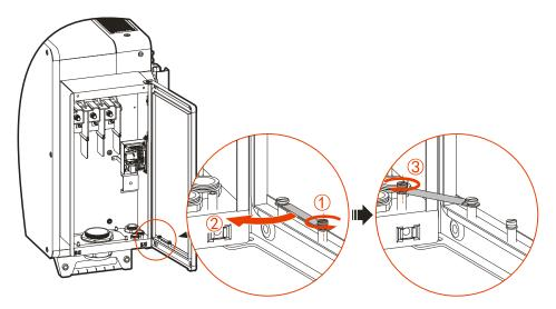
Figure 3-31 Operation diagram of limiting lever
