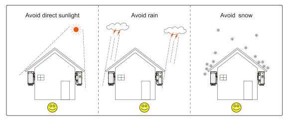
Figure 3-3 Recommended installation location
