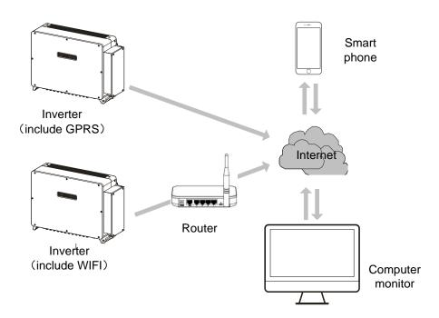
Figure 2-13 WIFI/GPRS monitoring solution
