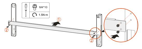
Figure 3-11 Assemble installation holder
