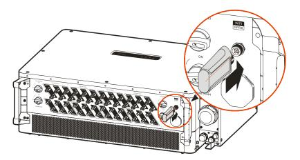
Figure 3-44 WIFI/GPRS communication connection
