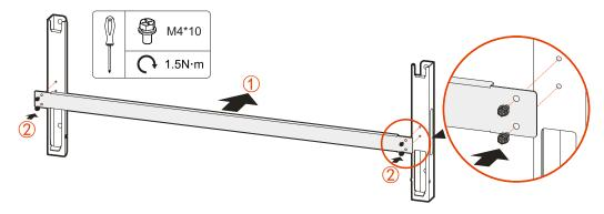
Figure 3-18 Assemble installation holder
