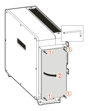
Figure 3-30 Open the wiring cover
