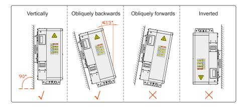
Figure 3-8 Illustration of installation method
