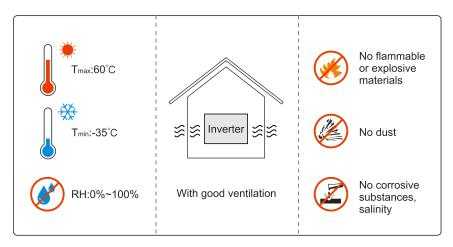
Figure 3-2 Installation environment requirements
