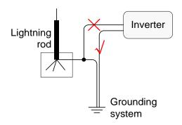
Figure 3-28 Grounding diagram of inverter
