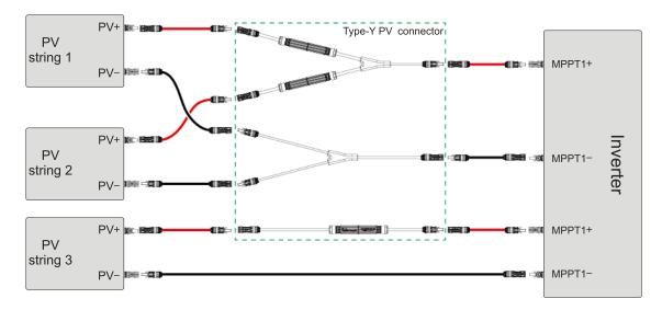
Figure 3-40 Wiring diagram (connected from PV string)
