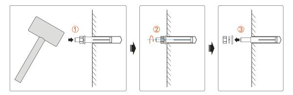
Figure 3-22 Expansion bolt installation diagram
